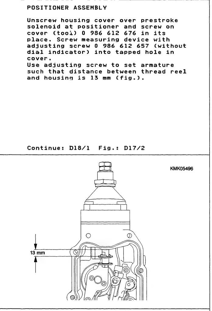
Note: On positioners as of end of 1994 the housing cover over the prestroke solenoid is provided as standard with the tapped hole for the measuring device and sealed with a screw plug. Cover replacement is then not necessary.
